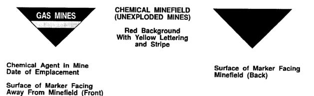
Figure 5-9. NBC Contamination Marking Signs.
